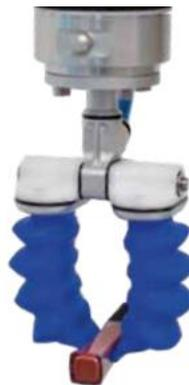
Figura 1.2 Pinza mGrip, Soft robotics
