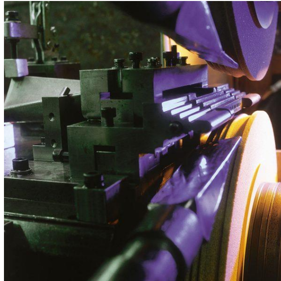
Figure 1.16. Creep feed grinding of a blade root [24].
