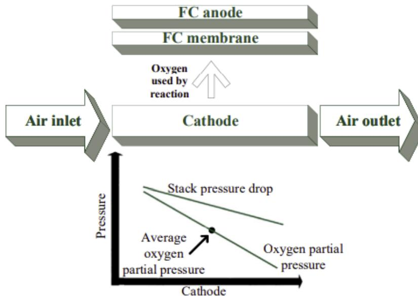
Figure 2.10: Schematic overview of the oxygen partial pressure drop inside the fuel cell stack
