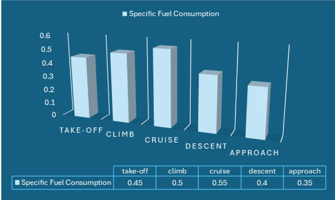
Figure 3.6: Specific fuel consumption for a Jet A1 CFM-56 [1/h]
