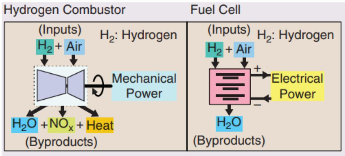
Figure 2.1: A comparison between the hydrogen combustor and the fuel cell conversion system, elucidating the inputs and outputs
