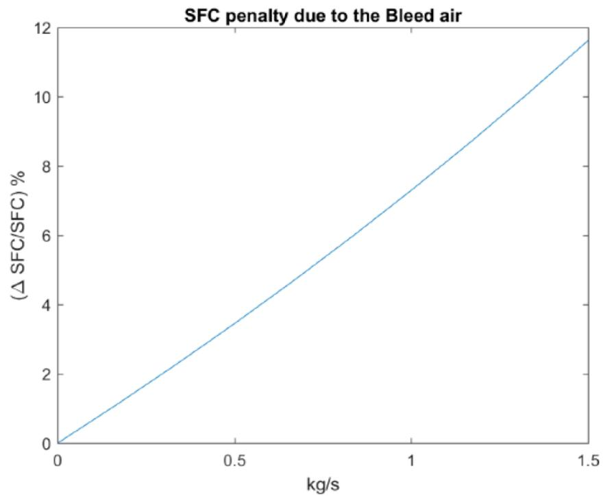
Figure 3.28: SFC reduction due to bleed
