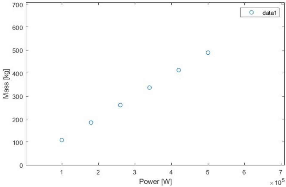
Figure 2.17: Variation of FC's mass in function of Output power
