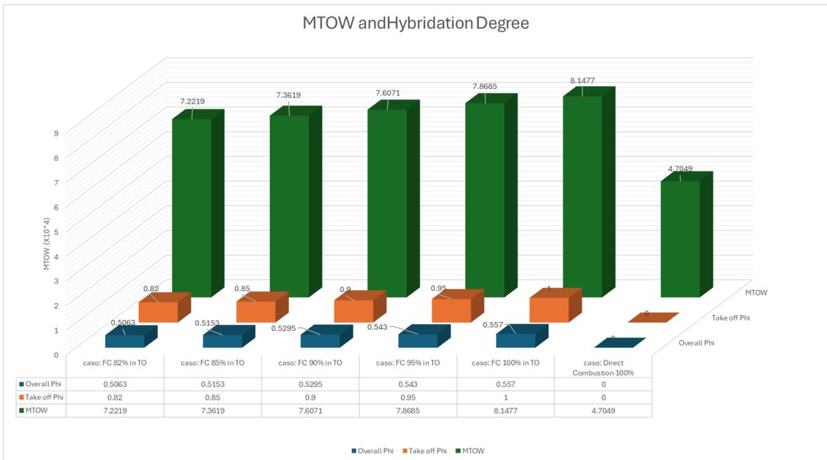
Figure 4.3: MTOW vs. Hybridation Degree
