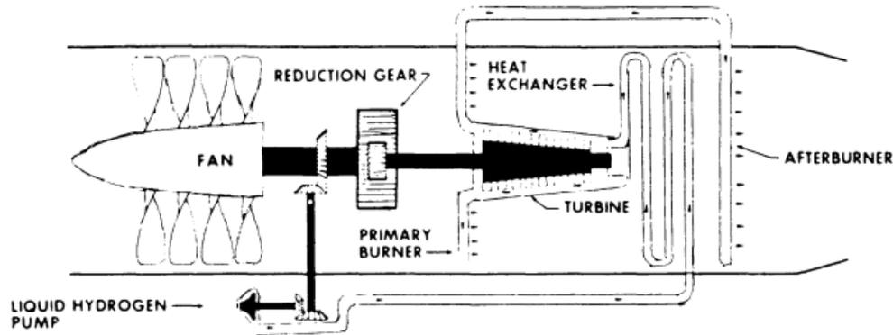
Figure 1.14: Model 304 engine
