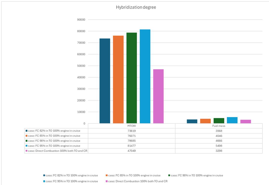
Figure 4.1: MTOW Comparison between direct combustion and fuel cell combustion
