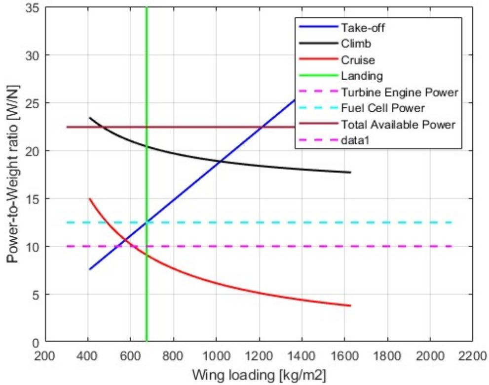
Figure 3.21: Matching chart: Fuel Cell 100 % active during take off
