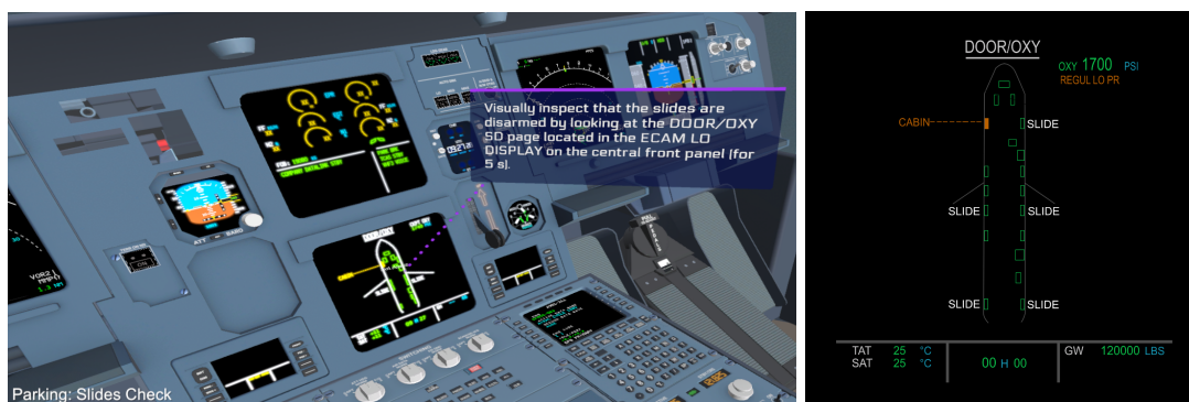
Figura 4.8: Nodo Slides Check Disarmed e schermata DOOR/OXY.
