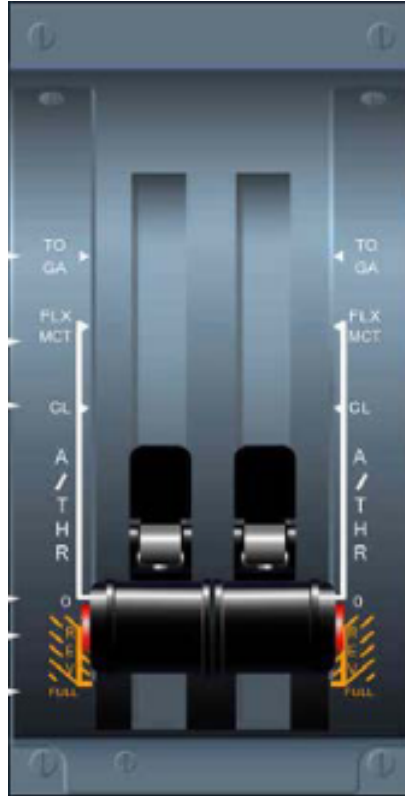
Figure 2.2: A320 thrust lever
