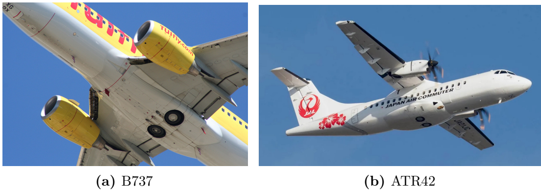
Figure 2.16: B737 and ATR42 main landing gear wheels in retracted position from [48]
