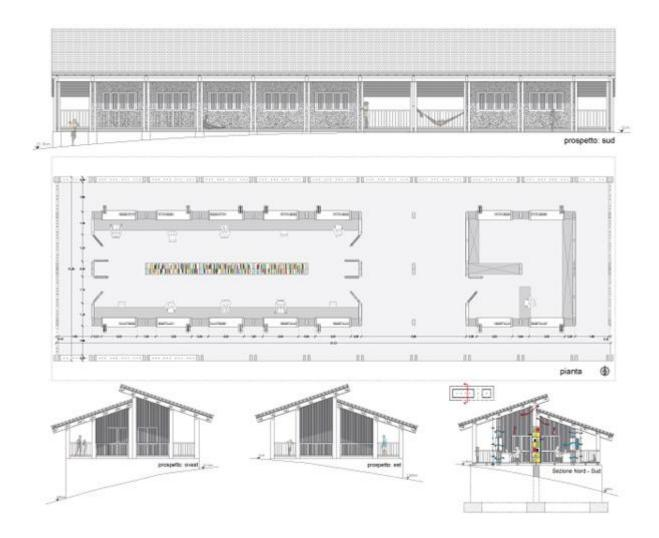
The materials and construction techniques are similar to those used in the Caracol House: wood for the structure and the finishing and concrete only for the foundations, in order to promote the use of local and recycled materials. In fact the wood used came from the trees falled for the construction of the airport realized by the company Pearl Island SA.
