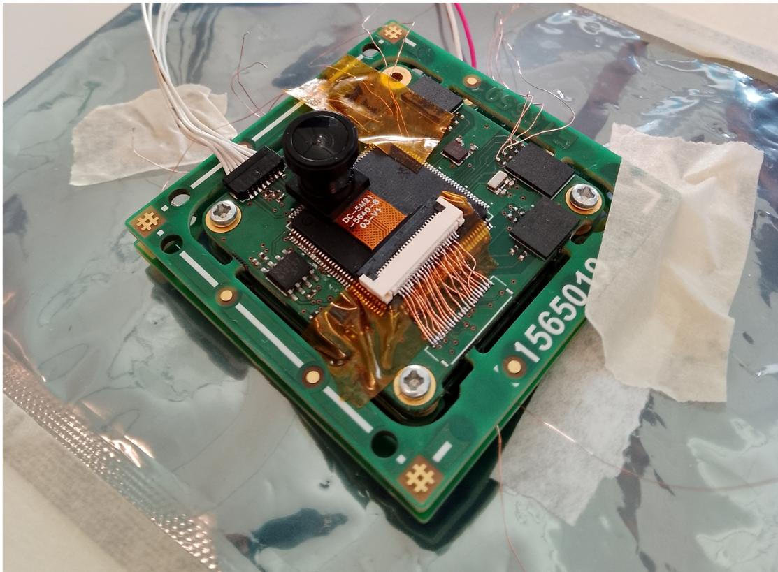
Figure 6.15: Image of the Development Model of the Delfi-TWIN imaging system during a performance test. The OV5640 test sensor is connected to the sensor control and data interface.
