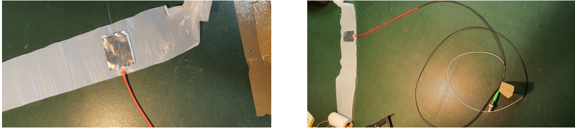
Figure 4.1: Packaging of FBG sensor for temperature tests in the climatic chamber
