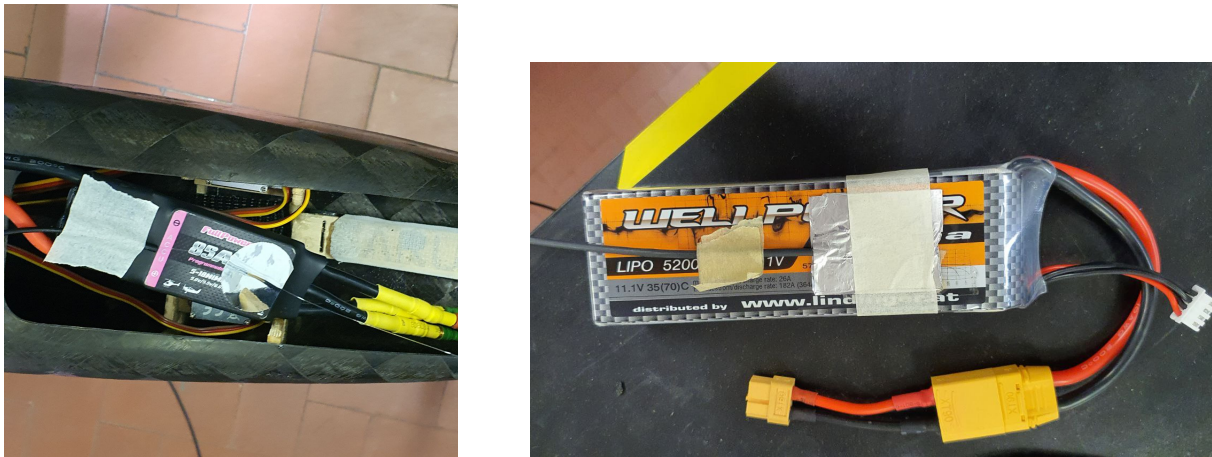
Figure 5.2: ESC and battery set-up
