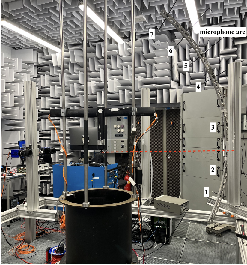
Figure 4.6: Microphone arc mounted in the A-tunnel.
