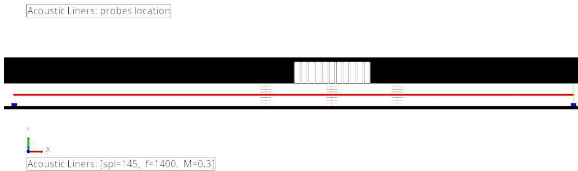
Fig. 3.14 Surface plane (probe plane), used for measurement of pressure along the duct axis.
