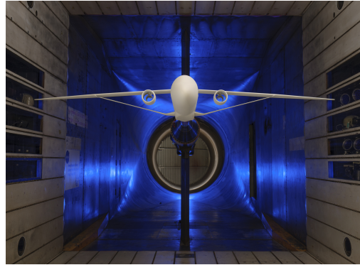
Fig. 2.1: Wind tunnel test of a scale model of a Truss Braced Wing configuration aircraft at NASA Ames Research Center. Source: NASA, 2023 [39] .
