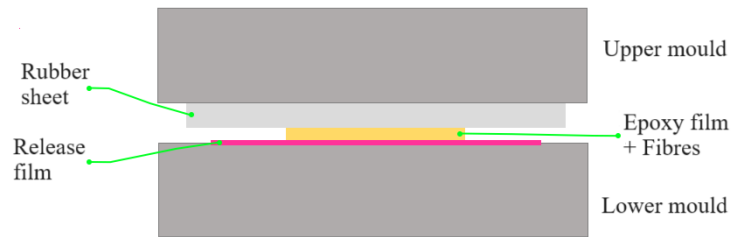
Figure 3.5: Hot pressing set-up.
