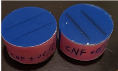
Figure 3.10: Specimens ready for microscopy, CNF+VE on left and CNF+E on right.
