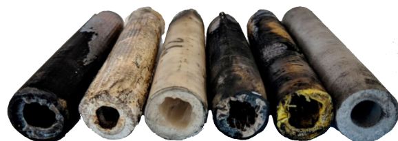
(b) After test, in order: ABS, PLA, PP, ASA, PETG, PLA-AI
