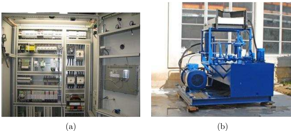
Figure 2.2: SHAKESPEARE shaking table ([33]): (a) shaking table control unit; (b) external hydraulic pumps that provide the hydraulic power for the shaking table facility
