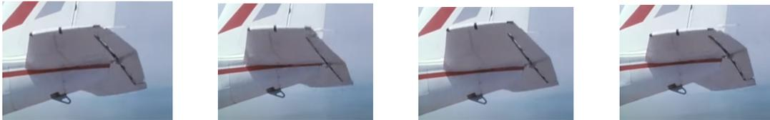
Figure 2.3: PA-30 Twin Comanche tail flutter test
