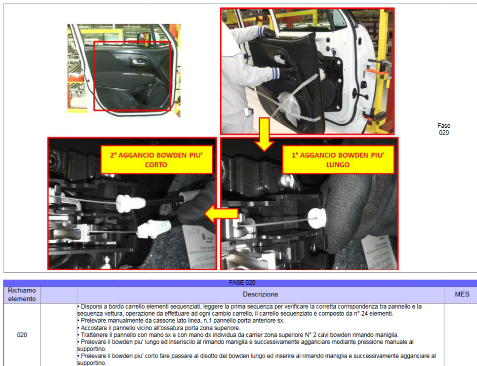
Figure 5.2. Operational card for manual labor in assembling the left front door panel
