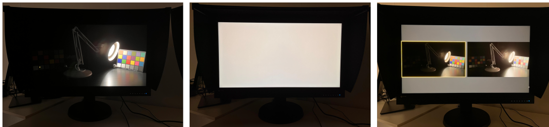
Figure 4.6: Experiment setup. The subject looks at the HDR image first. Then a gray scale image is projected for an adaptation time for the eyes. Finally, the subject is asked to express a preference between 2 options and for 6 times for each test image.
