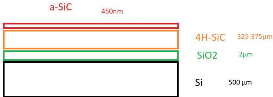
Fig. 26: Graphical description of the sample used to perform laser annealing for the whole work thesis duration.
