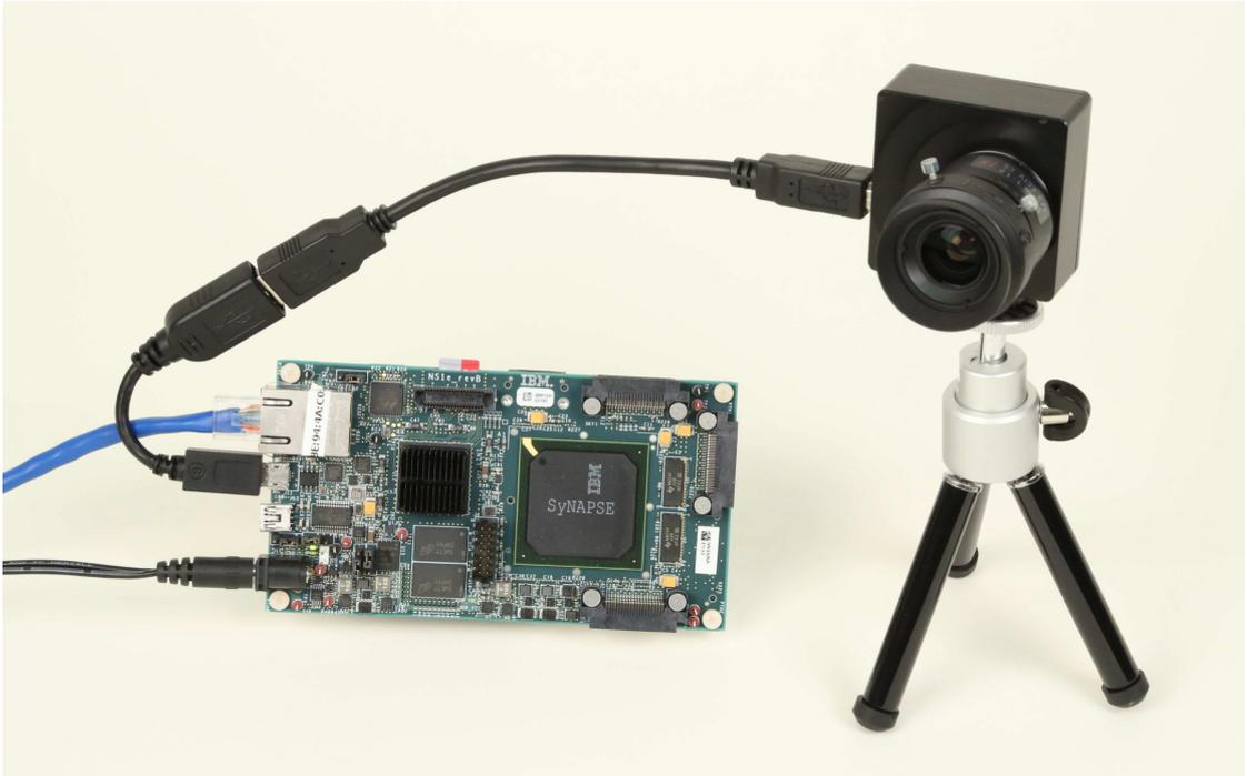
**Figure 11.6:** In the figure can be seen the hardware setup used to record the DVS dataset. There is a iniLabs DVS128 camera (128x128 pixel Dynamic Vision Sensor) capable to generate events when a pixel value changes magnitude by a user-tunable threshold. In addition to the spatial coordinates, the event encodes the timestamp indicating when the spike was registered. [65]
