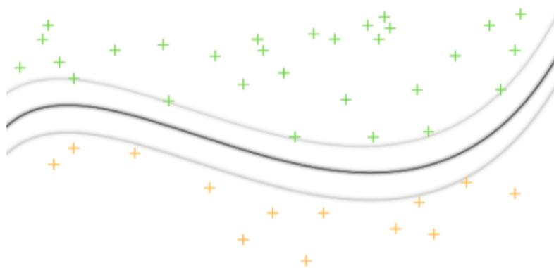
**Figure 4.6:** Example of a result of an SVC classification. The green points correspond to one class and the orange ones to the other class. The black line is the hyperplanes and the gray lines are the margins
