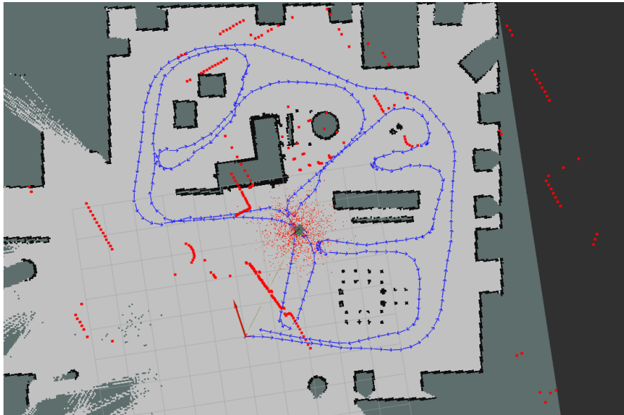
Figure 3.9: Rough estimated pose has been initialized as the centroid of the cluster and a set of particles has been generated around it
