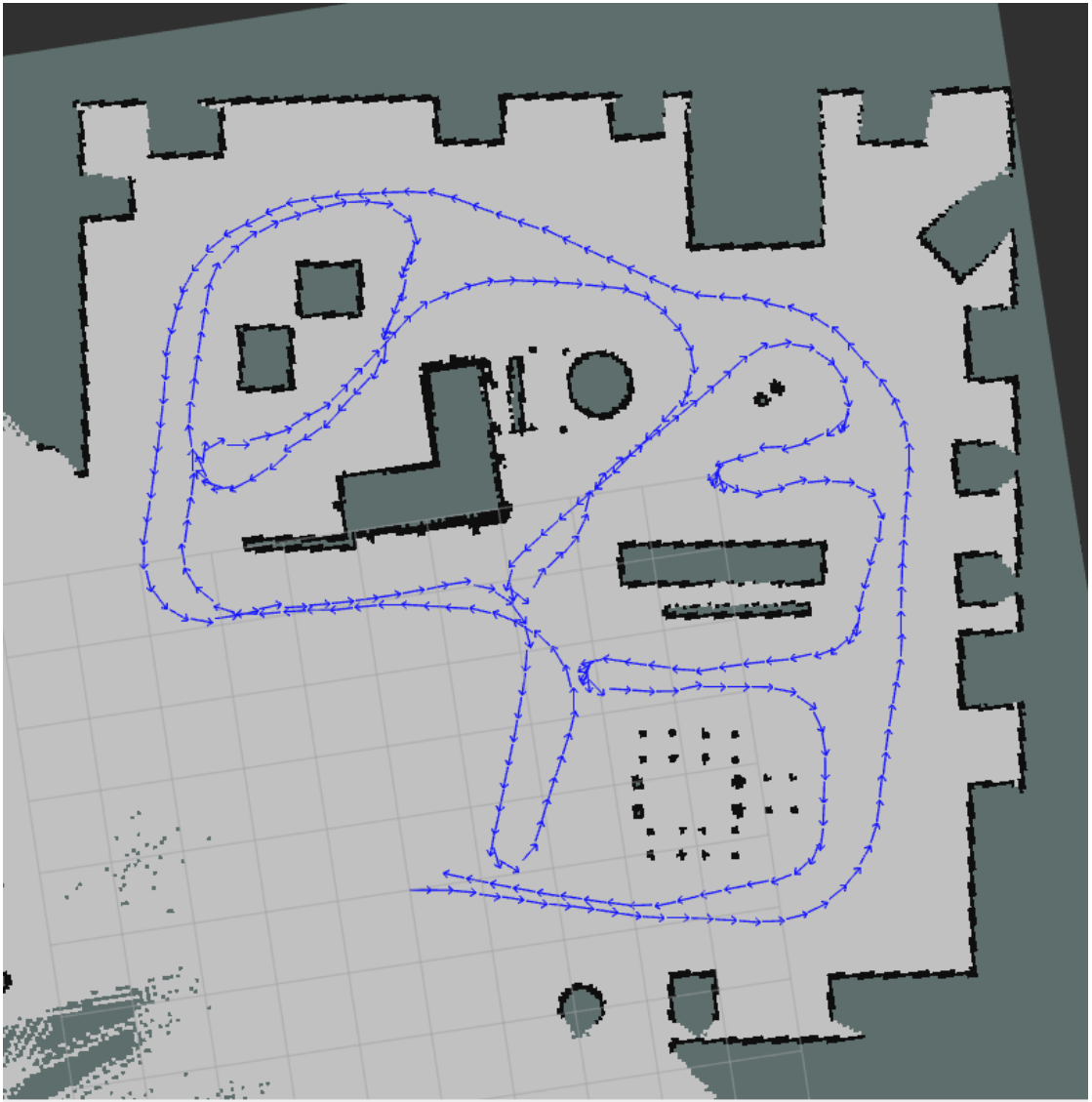
Figure 3.3: Sparse image database created with the ROS2 node. The blue arrows represent poses at which the images were taken.
