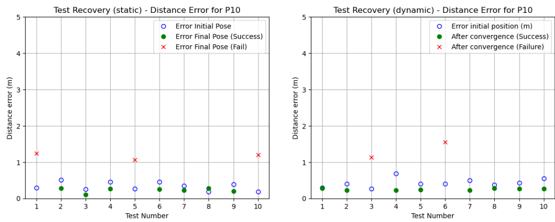
Figure 5.12: Distance error in position 10 in static and dynamic scenario
