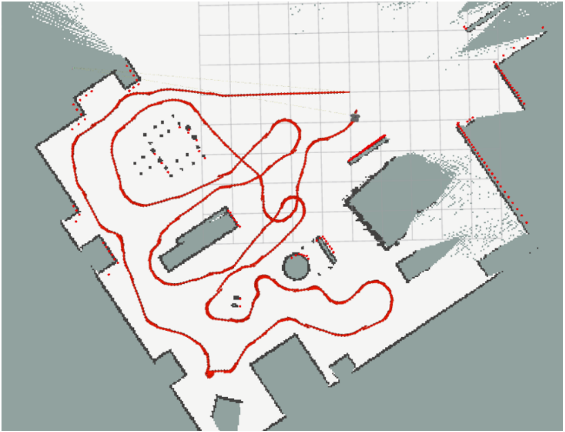
Figure 3.2: Dense image database created with the ROS2 node. The red path is composed of poses to which images are associated.
