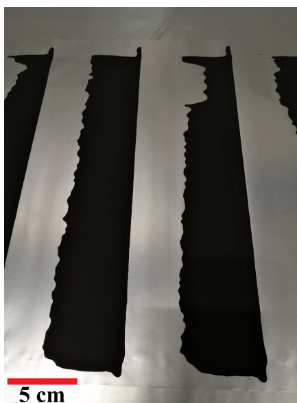
Figure 5.5: A R2R coating made with the most liquid slurry. As shown, the coating didn't go well, due to slurry slipping on the bottom.
