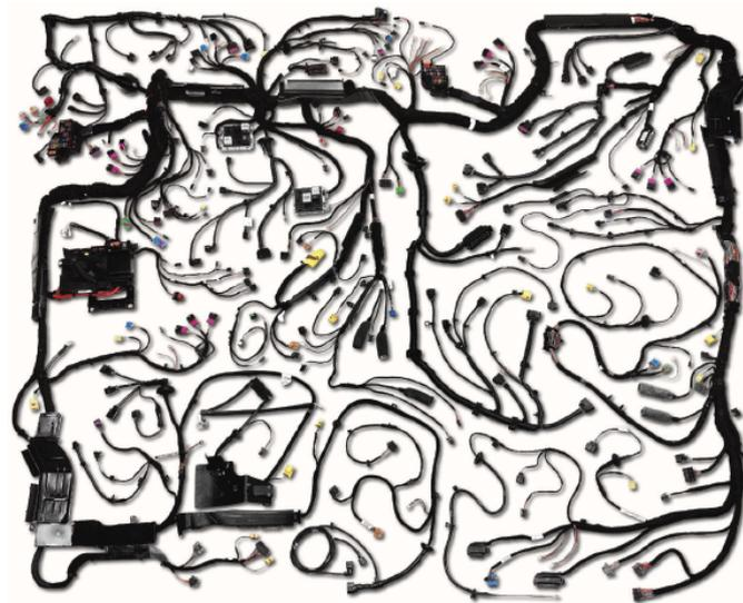
**Figure 1.3:** Wiring Harness, source:[6]
