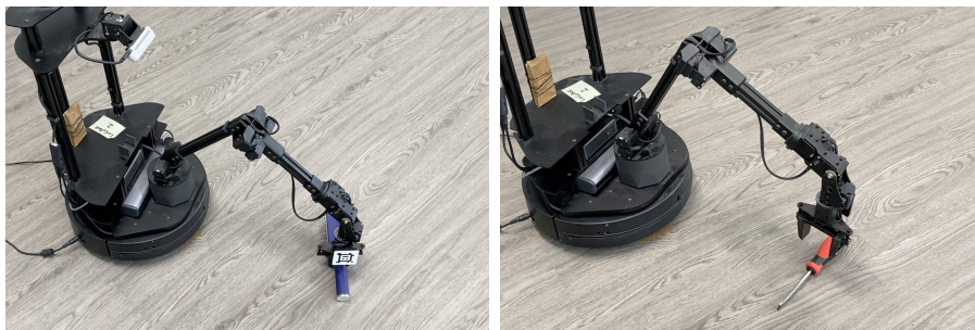
Figure 9.10: Different gripper orientations for different object poses.
