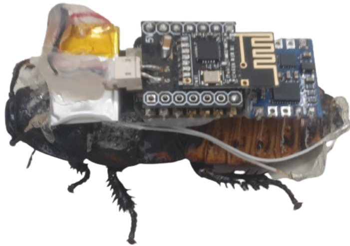
Fig. 2.2 MHC that has undergone surgery on both antennae and cerci
