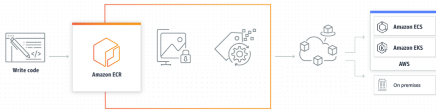
Figure 4.6. Example of how Amazon ECR works in production and for pulling images [9]
