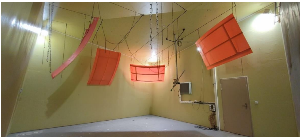
Figure 7: The reverberation room at KU Leuven
