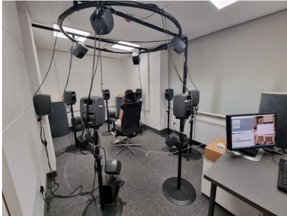
Fig 28-29: an immersive test in Audio Space Lab (left); orders of ambisonics (right).
