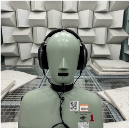
Fig 36-37: playback volume adjustment in anechoic chamber (left); Sennheiser HD650 frequency response (right).
