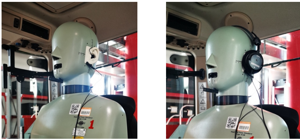
Fig 34-35: B&K 4101 microphone headset position inside the ear (left); Siemens ABH04 microphone headset position outside the ear (right).
