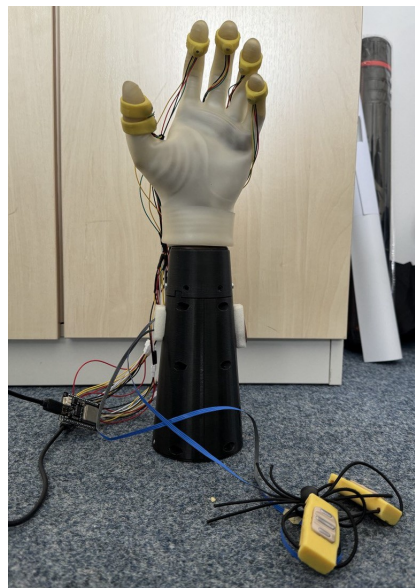
Figure 5.8: Sensors' placement in the final design of the robotic hand. Each fingertip is equipped with a single sensor, except for the thumb, where two sensors are positioned to enhance force measurement accuracy, considering the thumb's frequent contact in various tasks.
