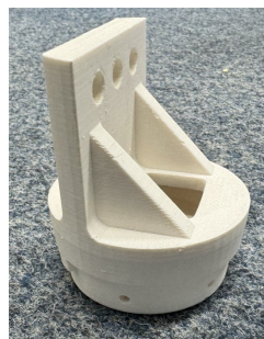
(b) Image of the 3D-printed support. ABS and QSR support materials were used.
