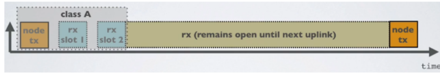
Figure 1.5: (LoRa Class-C) Bidirectional end devices with maximal receive slots timing of end device timing of transmission/reception cycle(Source [2]).
