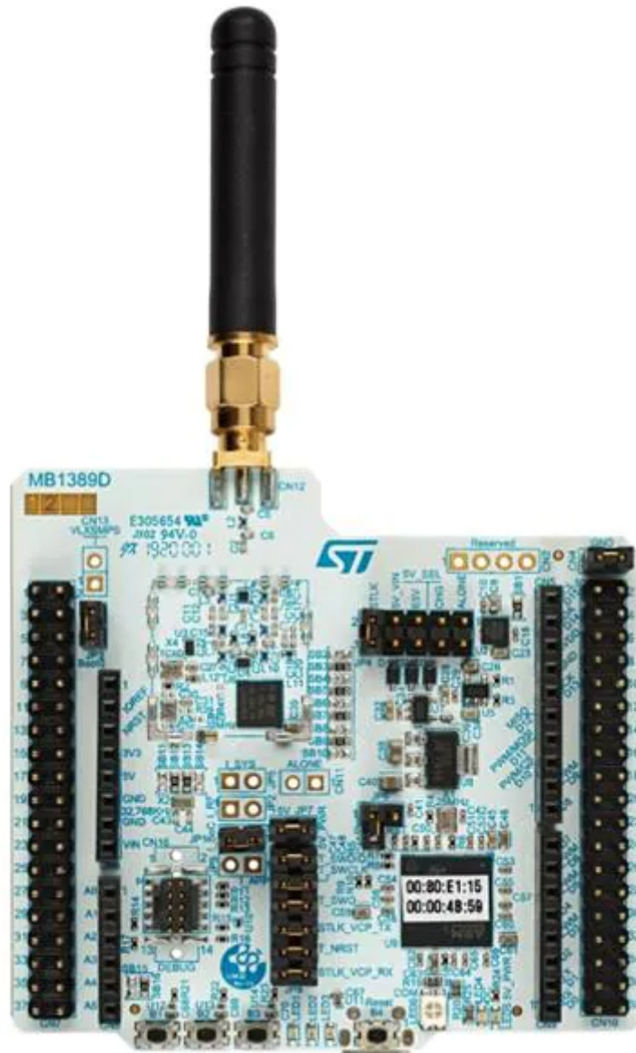
Figure 2.5: STM32-WL55JC1 Nucleo Board from STMicroelectronics (Source [4]).
