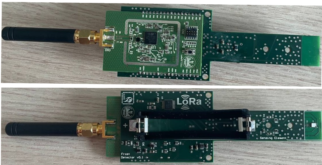
Figure 7.13: Top view and Bottom view of the Frost Detection System assembled.
