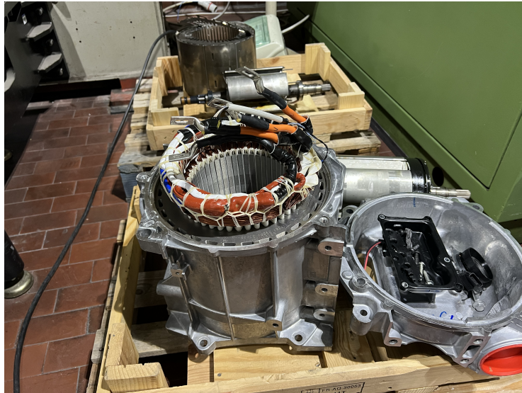
Figure 6.1: Machine under test, Renault ZOE 135 WFSM.
