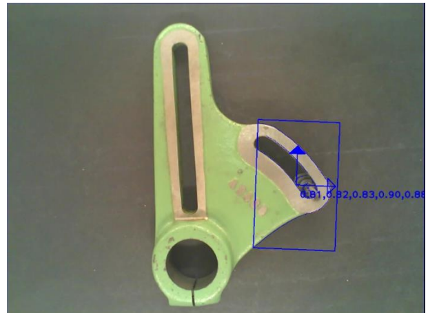
Figure 21: Object detection (rotated part)
