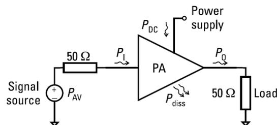
Figure 2.3: Power flow in a PA [3]
