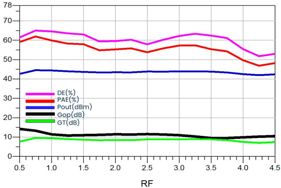
Figure 3.24: HB simulation results at 35 dBm of input power versus Frequency for circuit schematic
