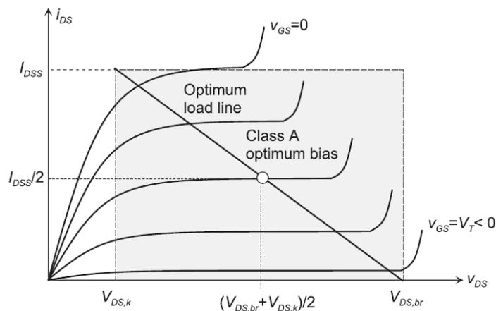
Figure 2.5: Load line of class A amplifier with optimum load [6]
