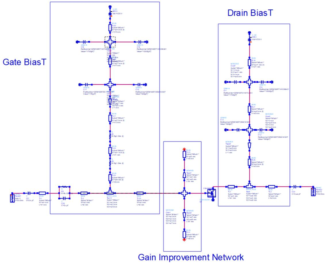
Figure 3.10: Schematic without the matching networks
