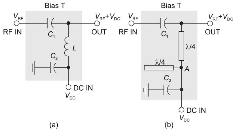
Figure 3.5: Lumped parameter (a) and Distributed parameter (b) of Bias Ts [6].
