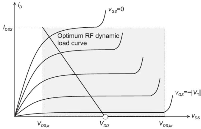
Figure 2.7: Load line of class B amplifier with optimum load [6]
