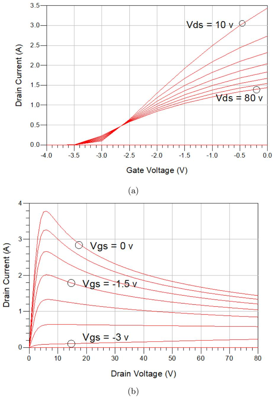
Figure 3.1: Trans-characteristics (a) and Output-characteristics (b) of the active device
