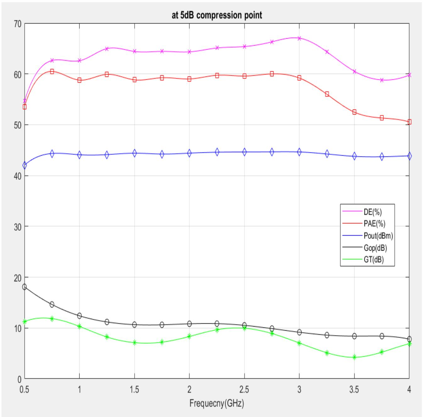
Figure 4.8: HB simulation results of the layout at 5 dB gain compression point using MATLAB
