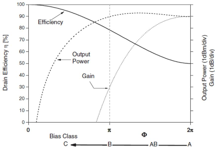
Figure 2.9: Tuned Load theoretical performance as a function of the drain CCA [12]
