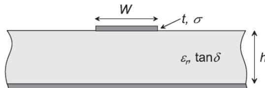
Figure 4.1: Cross-section of a microstrip line [6]
