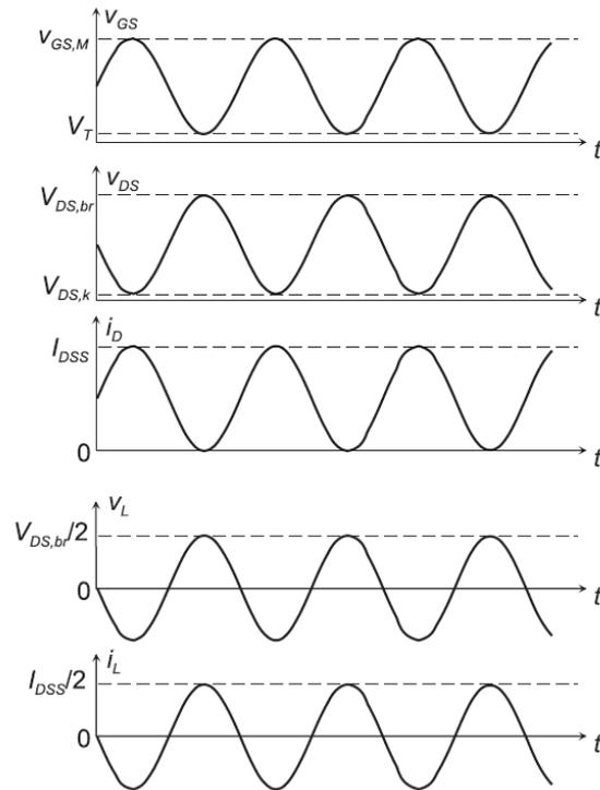
Figure 2.6: Waveforms of a class A amplifier [6]
