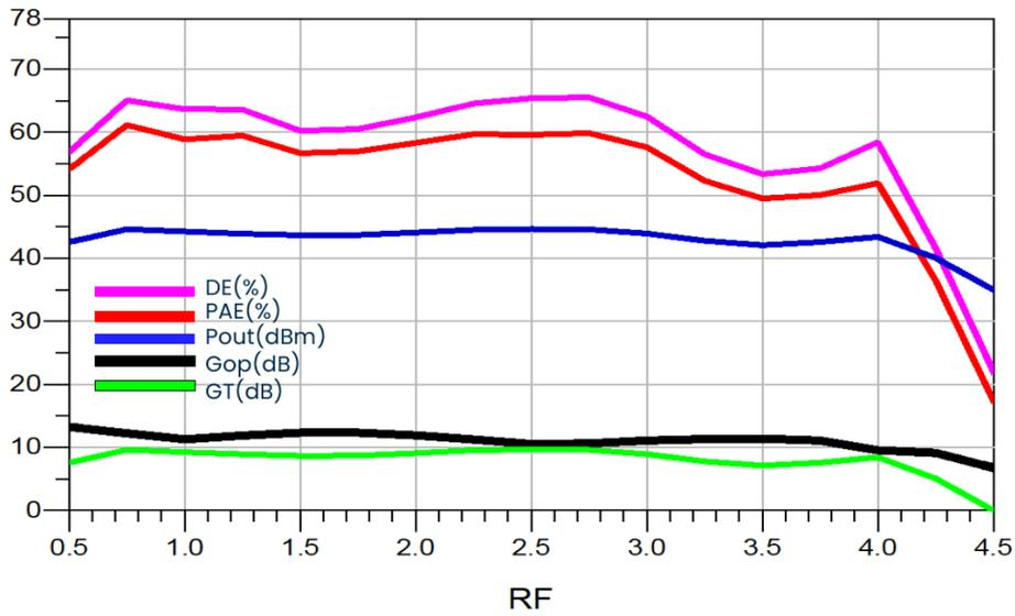
Figure 4.7: HB simulation results at 35 dBm of input power versus Frequency for circuit layout
