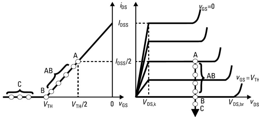
Figure 2.4: The transfer characteristics (a) and output characteristics (b) of an ideal FET vary according to different bias point classifications [3].
