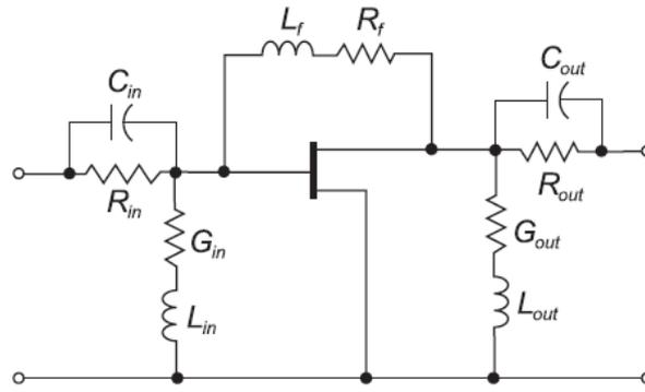
Figure 3.2: Stabilization network [6]
