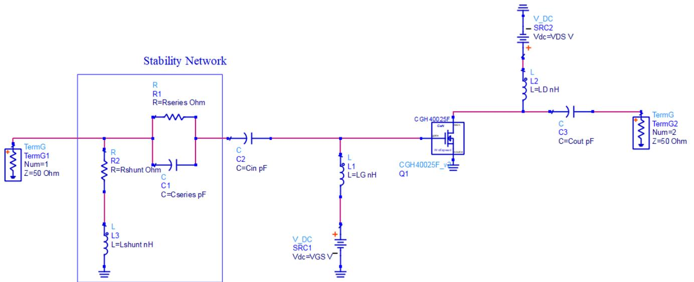
Figure 3.3: Stabilization network with ideal bias
