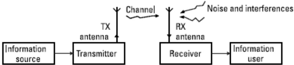
Figure 2.1: Transmitter and Receiver in Communication Systems [3]
