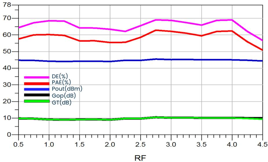
Figure 3.14: HB simulation results at 35 dBm of input power versus Frequency
