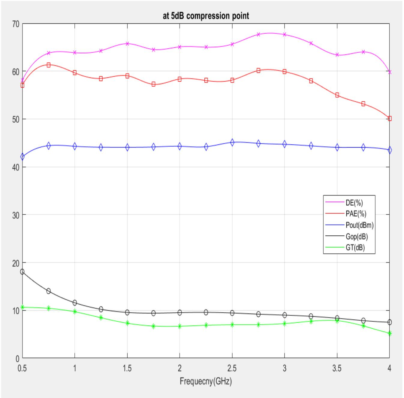
Figure 3.25: HB simulation results at 5 dB gain compression point using MATLAB
