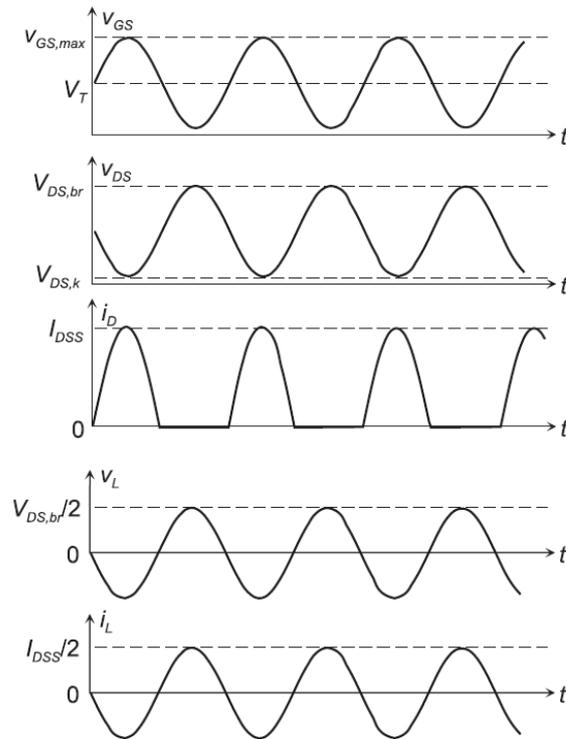
Figure 2.8: Waveforms of a class B amplifier [6]
