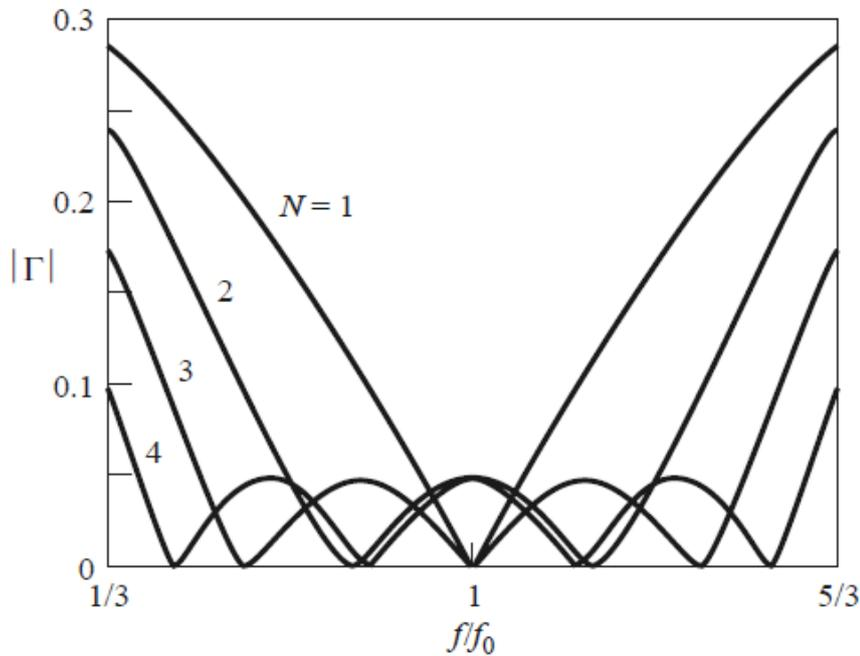
Figure 3.15: Reflection coefficient magnitude versus frequency for the multi-section transformers [14]
