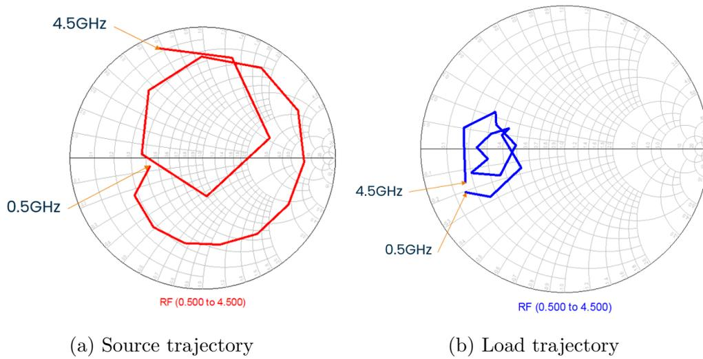
Figure 3.12: Optimum termination trajectories
