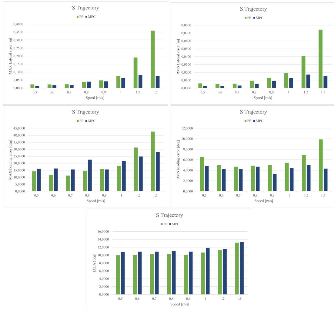
Figure 7.12: Comparison of controllers performance in experimental tests with S trajectory at different vehicle velocities
