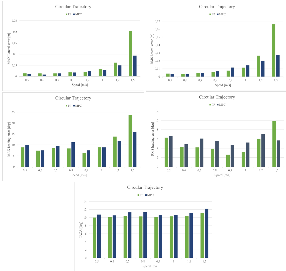
Figure 7.14: Comparison of controllers performance in experimental tests with circular trajectory at different vehicle velocities
