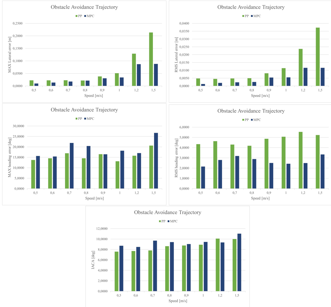
Figure 7.13: Comparison of controllers performance in experimental tests with eight trajectory at different vehicle velocities
