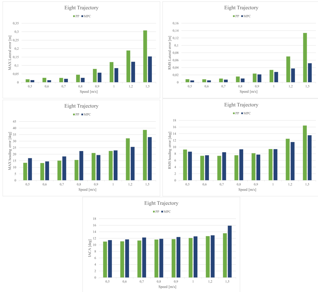
Figure 7.15: Comparison of controllers performance in experimental tests with eight trajectory at different vehicle velocities
