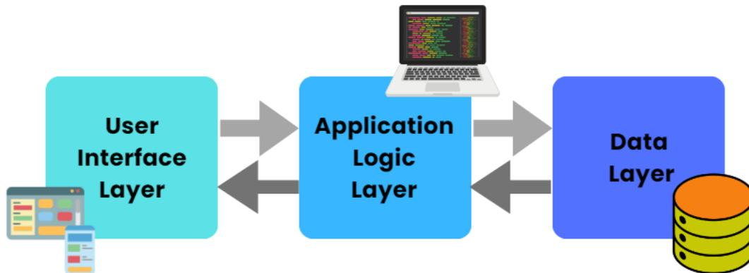
**Figure 7:** Layered architecture of LC-Neurorehab.
