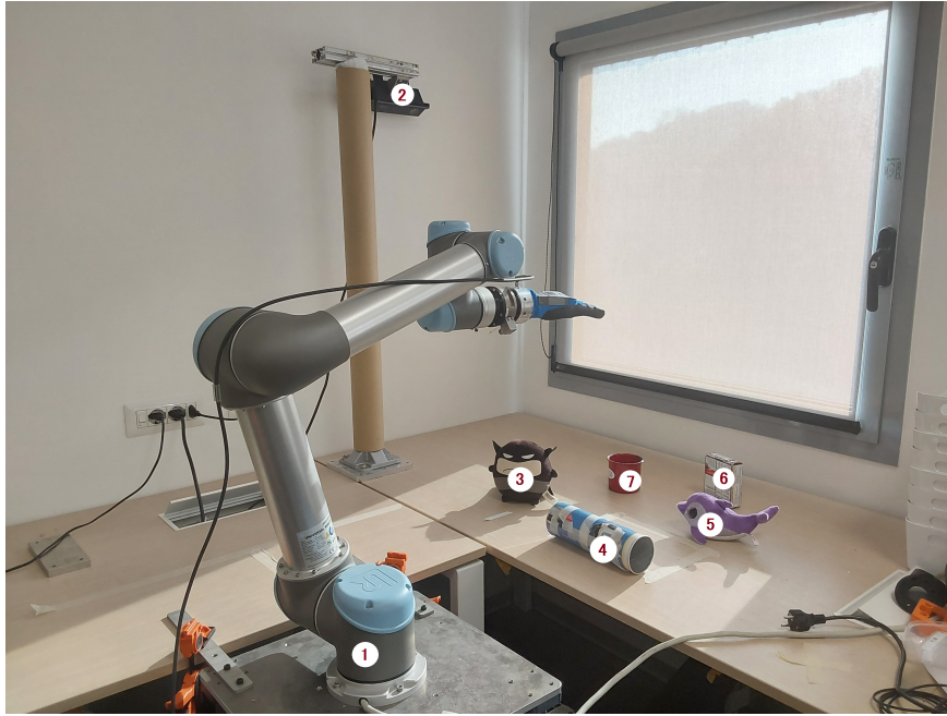
FIGURE 5.4: Real Experimental Setup. Ur5 robotic arm (1), Kinect Two RGB-D camera (2) and the Objects are indicated with IDs
