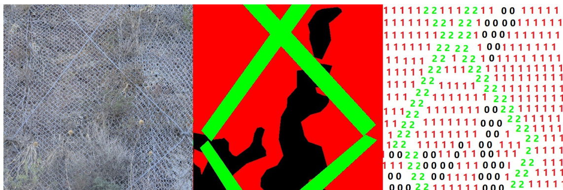
Figure 3.18: Pixel labeling is demonstrated; Original image in the left, ground truth mask in the center and corresponding pixel label in the right.
