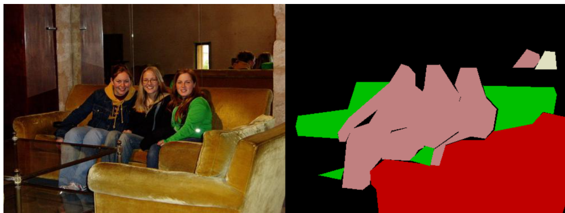
Figure 3.2: Semantic segmentation mask creation is demonstrated with its corresponding image after annotations done by LabelMe[22].
