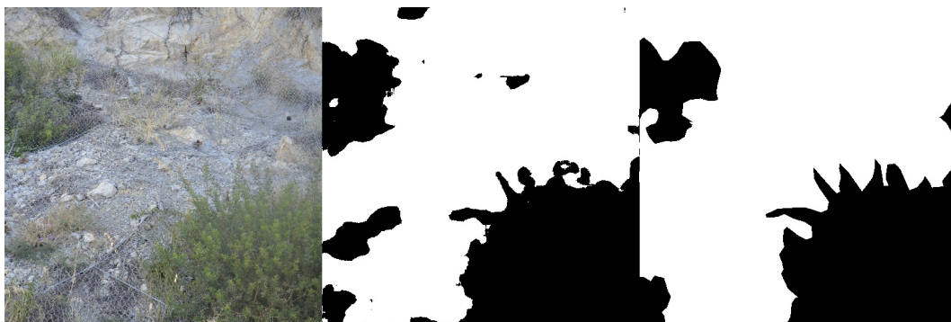
Figure 3.16: A sample of mesh prediction that is trained by U-Net++ model on input images that is utilized with augmentation techniques. Input image in the left, prediction in the center and target mask in the right.
