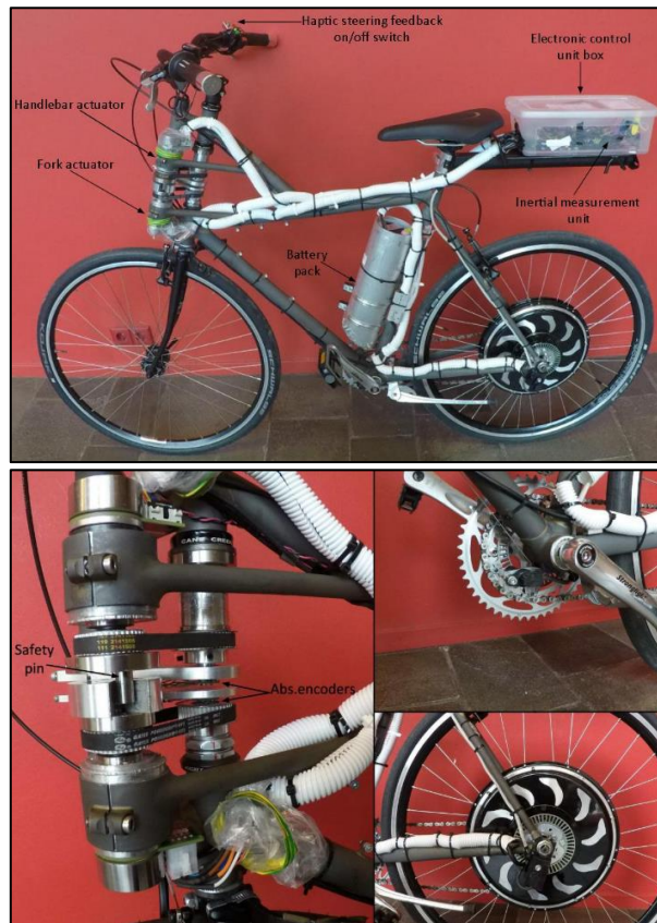
Figure 6: Steer by wire bicycle prototype and system close up.
