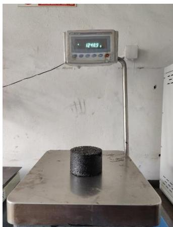
**Figura 49.** Pesatura in aria  $m_1$ .
