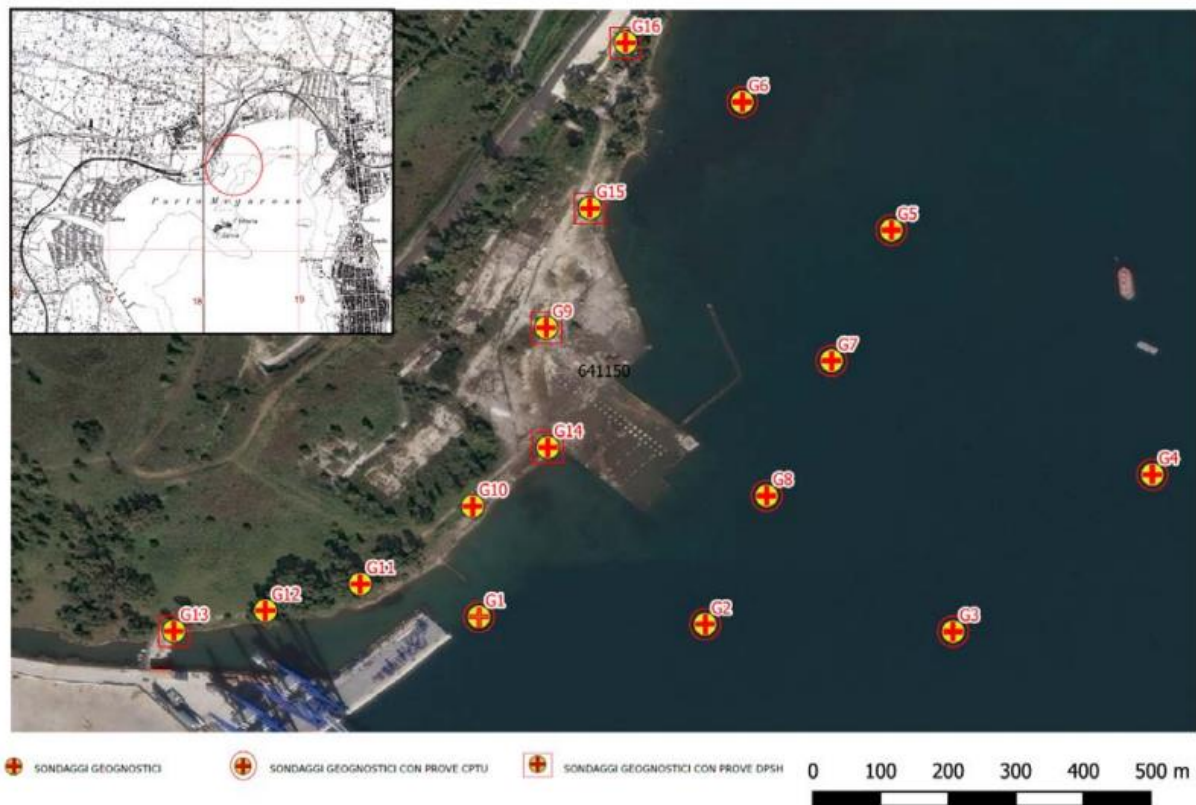
Figure 5.1 Plan with the location of the CPTU and DPSH surveys and tests
