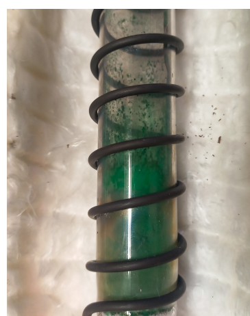
(c) Heating wires.
