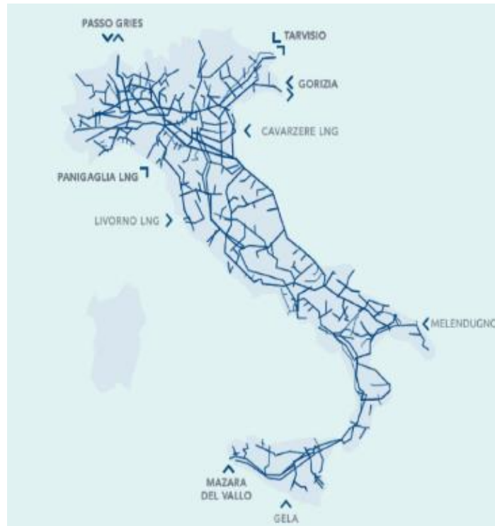
Figure 1.9 - Snam gas transmission network scheme [12]
