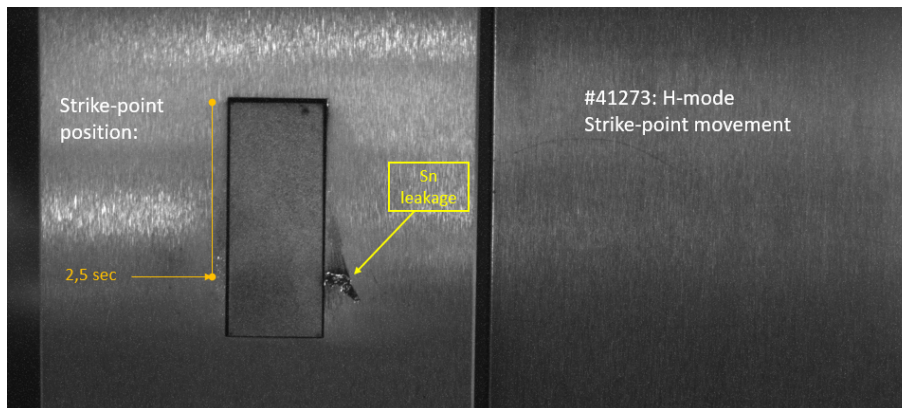
Figure 43: CPS image #41273 discharge strike-point. Presentation: "Performance of a liquid tin divertor target during ASDEX Upgrade L and H-mode operation", authors: "J.G.A. Scholte, B. Boeswirth"
