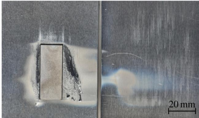
Figure 2.6: LTM with adjacent TZM (left) and W (right) divertor tile after exposure [6]
