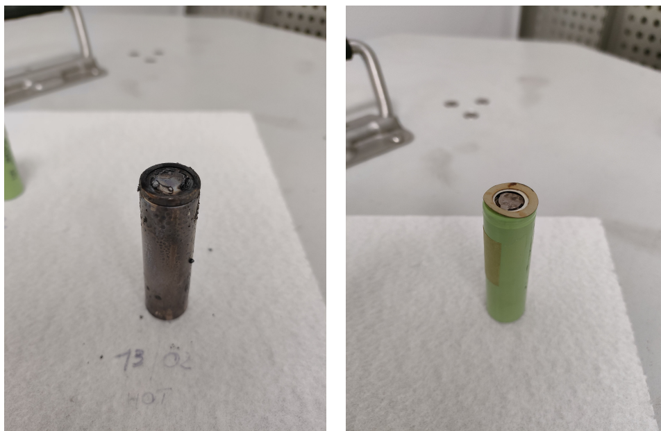
Figure 56: LG cell overheating (left) Samsung cell overheating (right)
