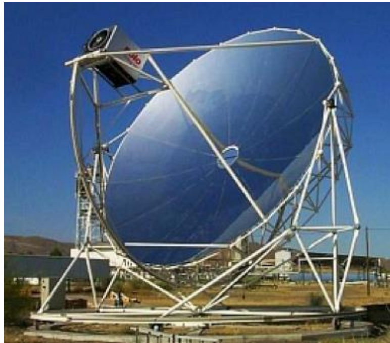
Figure 1.17: Schematic image (a) [16] and real image (b) of a parabolic dish collector [17]
