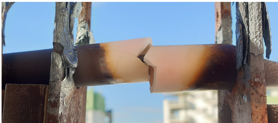
Figure 4.7: The fracture reported in the Alumina Receiver
