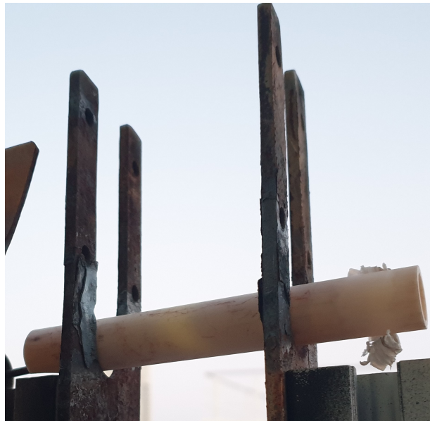
Figure 4.3: Alumina cylinder positioned at the focal point
