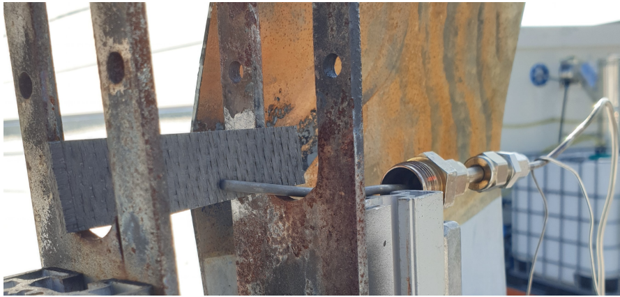
Figure 4.12: The black ATL SiC Receiver with the positioned Thermocouple
