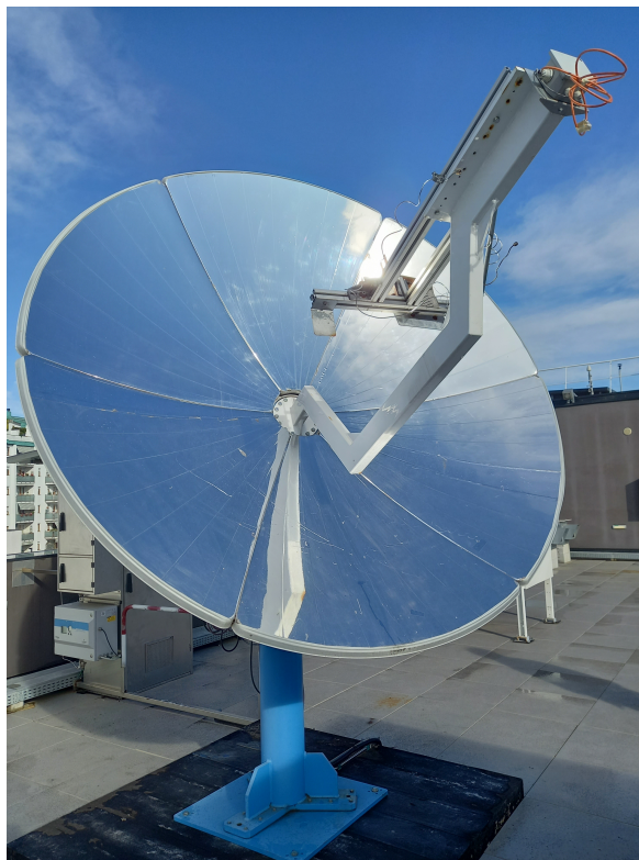
Figure 4.1: Solar parabolic dish on the Energy Center
