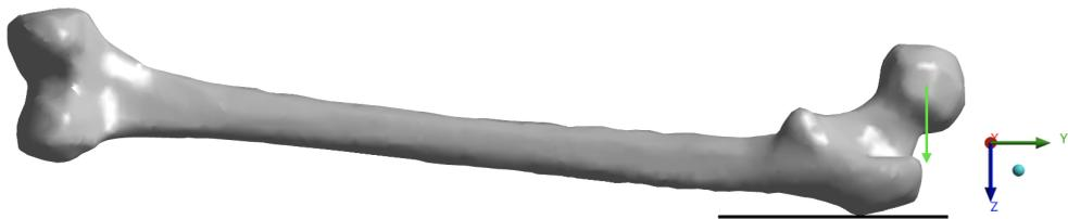
**Figure 2.4:** Load condition for the *reference case*: load force applied to the centre of femoral head (green arrow).
