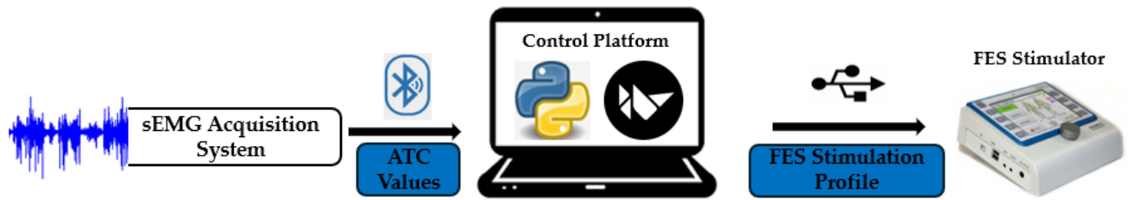
Figure 3.1: System Overview: the hardware part is composed of the sEMG acquisition system and the electrical stimulator. The acquisition devices communicate via Bluetooth with the control platform, while the stimulator uses a USB cable for the connection.
