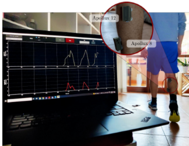
Figure 3.3: Real-time acquisition using Apollux devices: two ATC profile extracted from Gastrocnemius Medialis and Soleus muscles [43]
